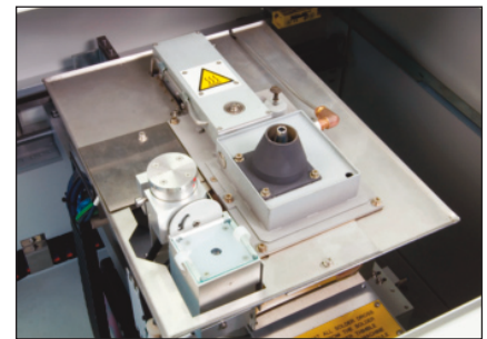
SOLDER BATH AND PUMP ASSEMBLY WITH DROP-JET FLUX HEAD AND PROGRAMMING CAMERA
