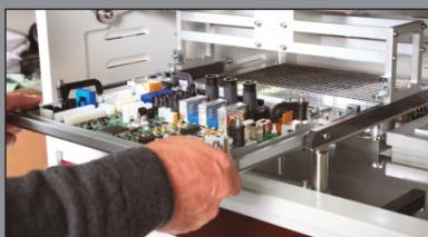
HANDLOAD QUICK CHANGE TOOLING CARRIER ASSEMBLY
